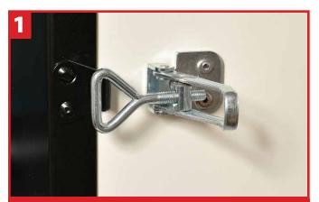
To access the cartridge filter, release the four toggle fasteners and unhook the front cover.
