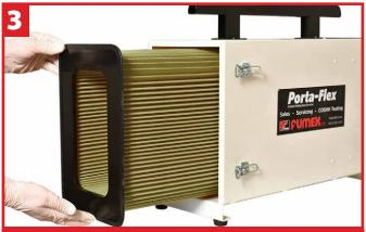
Slowly withdraw the old filter horizontally and place in a plastic bag and then seal the bag with tape. NB. Old filters must be disposed in accordance with Local Authority Guidelines.
