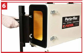
Refit the front cover and then reattach the four toggle fasteners to secure it in place. The extractor is now ready for use.
