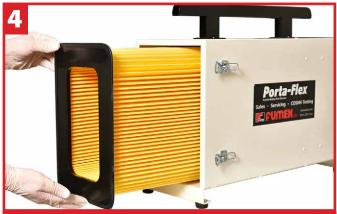
Install a new Fumex cartridge filter into the extractor. Using non-genuine filters will void the Porta-Flex warranty and may have a detrimental effect on efficiency.
