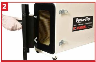
Carefully remove the front cover and combined spark trap. Check the spark trap, by removing the two wing nuts and clean if required.
