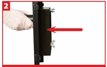
Carefully remove the front cover and combined spark trap (arrowed). To check the spark trap, remove the two wing nuts and clean if required.
