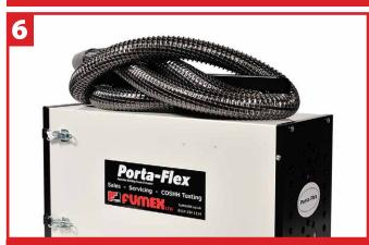
Disconnect extraction hose from both the nozzle and unit. The power supply cable and extraction hose can be wound around the carry handle for storage.
