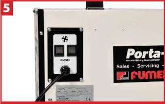
On completion of welding, turn off the Porta-Flex and disconnect the power supply cable from the socket.
